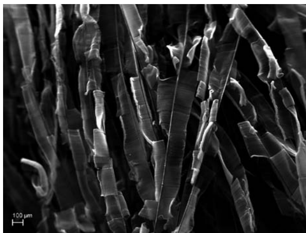
Figure 2. Aligned carbon nanotubes synthesized in the surface of structural fibres. This material is commonly known as fuzzy fibre.
