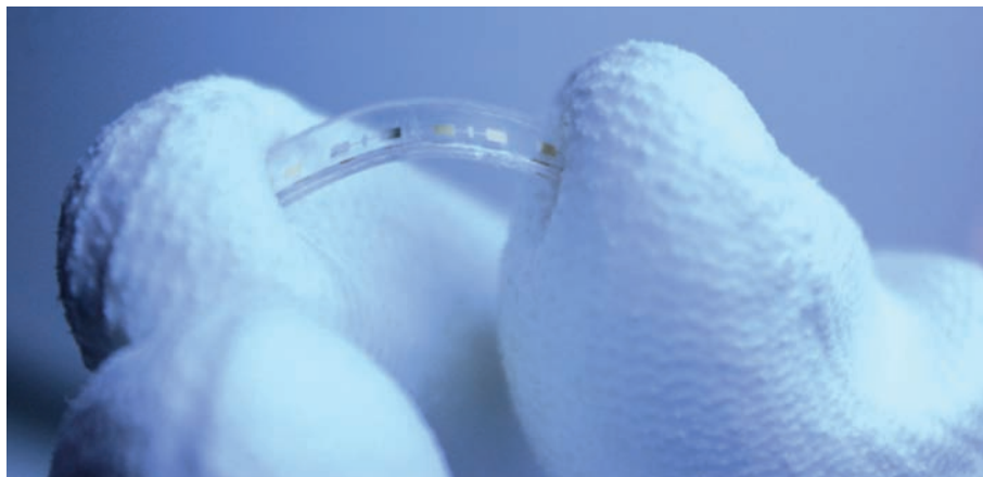
Picture of a flexible and quasi-transparent solar cell fabricated with two-dimensional semiconductors.
