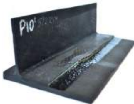
Figure 9. Detail of a stringer-skin integration manufactured by resin transfer moulding RTM.
