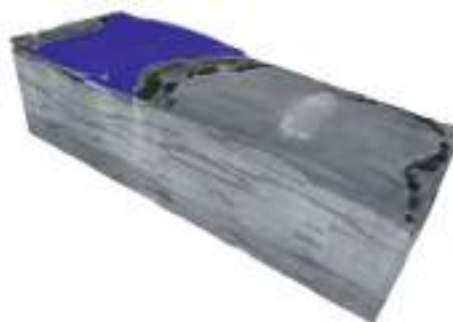
Figure 2. 3D X-ray tomography of an energy-storing structural composite.
