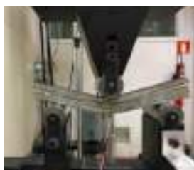
Figure 1. Fiber metal laminate (steel and glass) manufactured by UPM subjected to three-point bending (courtesy of Prof. Suárez Bermejo).
