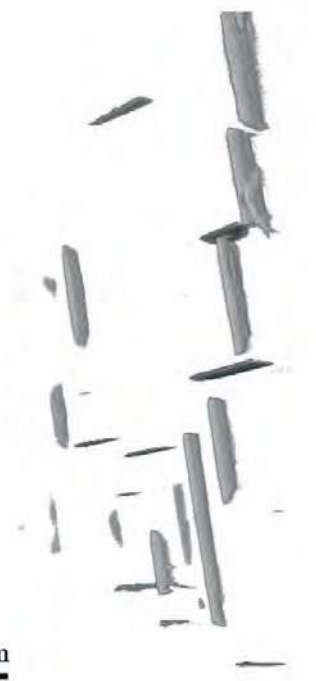
Precipitates, growing along a dislocation line, in an Al-Cu alloy (3D-TEM).
