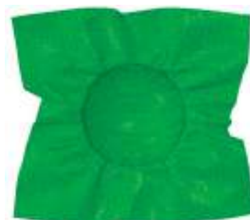
Figure 3. FEM deformation of a square fresh prepreg sheet during forming using and spherical indenter.
