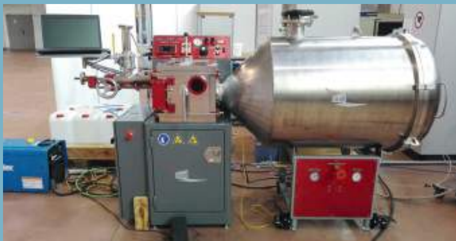
Figure 1. Gas atomizer unit available at IMDEA Materials.
