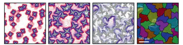
Figure 3. Multiscale simulation of crystal growth in an Al-10wt%Cu alloy, undercooled by 10°C below its liquidus temperature, in the presence of gravity-driven buoyancy. Time snapshots (left) show the growing crystals (black) and the Cu concentration field (blue-to-red). The final microstructure (right) exhibits irregular grain boundaries (black) and Cu-segregated regions (white). [Computational Materials Science 162, 206-227, 2019]
