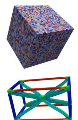
Figure 1. Up: Polycrystaline model containing 120.000 grains and 16.10<sup>6</sup> voxels. Down: Deformation of lattice structure, 2.10<sup>6</sup> voxels
