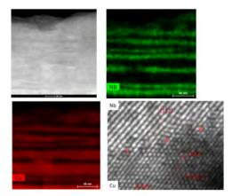
Figure 1. TEM images of a Cu/Nb nanolaminate, showing the Cu and Nb layers and the interface at atomic resolution.
