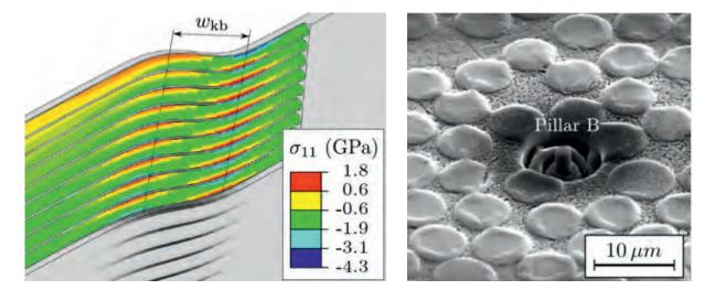
*Figure 3. a)* FIB milled pillar carved on carbon fibres. Pillars are submitted to compressive load to evaluate the mechanical properties, b) Simulated stress fields in a kink band formed under fibre compressive loads.
