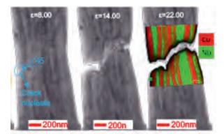
Figure 2. Snapshots taken at different stages of deformation and fracture of a specimen loaded parallel to the layers.
