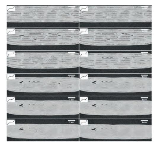
Figure 4. Time sequence as obtained from XCT in the same slice during the curing process of an Out-of-Autoclave composite material. The inset indicates the curing conditions (temperature and time).
