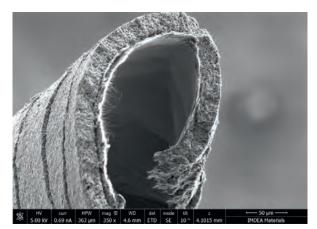
Figure 2. Electron micrograph of a lithium ion battery electrode with carbon nanotube fibre fabric current collector. The composite electrode has 60% higher specific capacity than commercial electrodes, retained even after fracture following tensile deformation above 15%.
