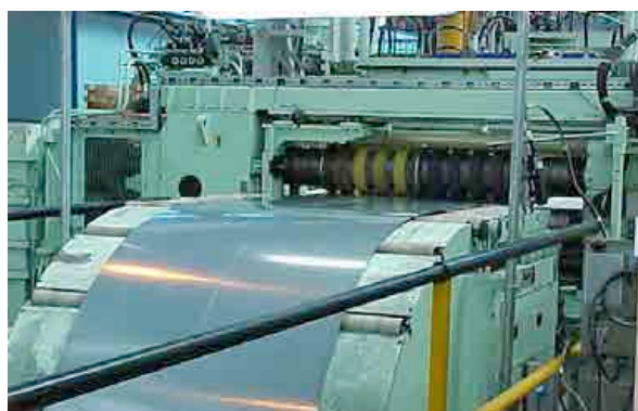
Figure 2. Slitting line (to make strips from the coil) for the final product (courtesy of ACERINOX).
