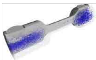
XCT: Porosity in die-cast Mg alloys
