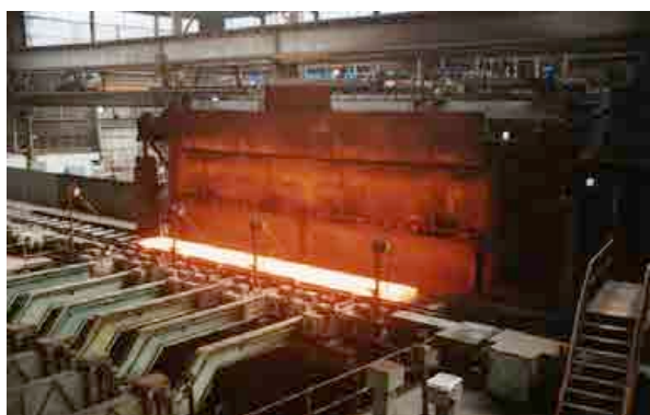
Figure 1. Exit of the furnace for re-heating of slabs in hot rolling (courtesy of ACERINOX).
