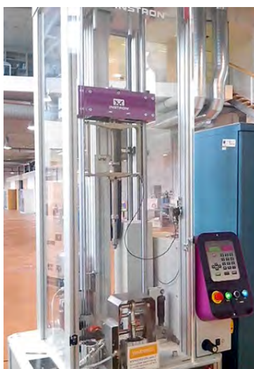
Figure 2. drop-weight testing frame with the sharp-tip metallic indenter to simulate ballast impact events.
