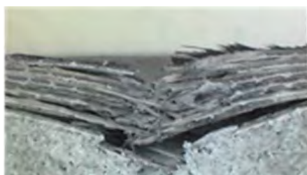
Figure 1. damages induced by simulated ballast impact on the carbon skin of a sandwich laminate for two different impact energy levels.
