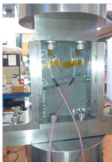
Figure 3. compression after impact strength evaluation.
