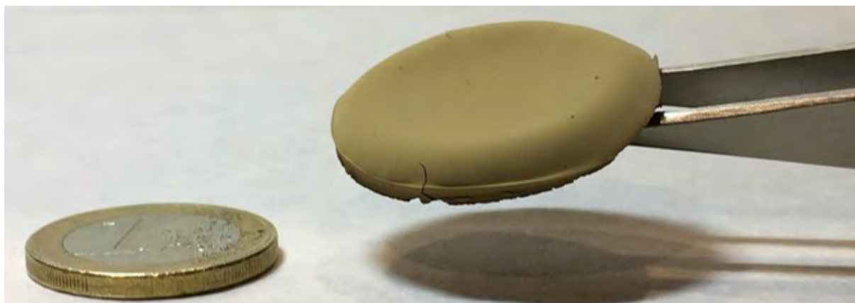
Figure 1: photograph of a freestanding anode of Si nanowires
