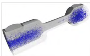
XCT: Porosity in die-cast Mg alloys
