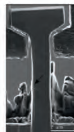
Micropillar compression / microtensile testing in SEM/TEM
