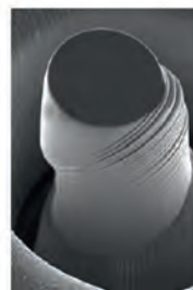
Micropillar compression / microtensile testing in SEM/TEM
