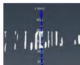
3D-TEM of Mg-Zn precipitates
