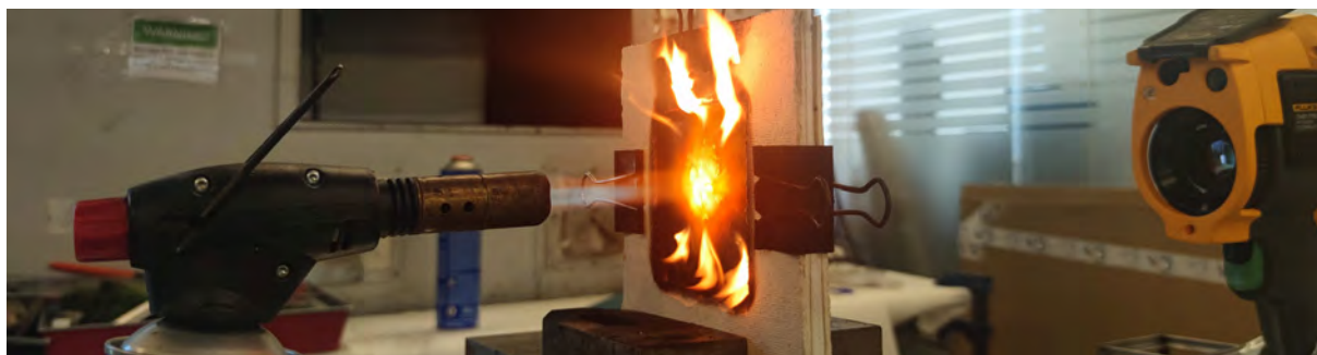
Screening of fire insulation properties of polymer composite panel with thermal camera
