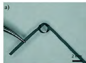
Schematic representation of an FCCVD reactor for generating silicon nanowires in the gas phase (left) and a photo of a stripe of self-standing silicon nanowire fabric showing its flexibility in terms of bending and knotting.
